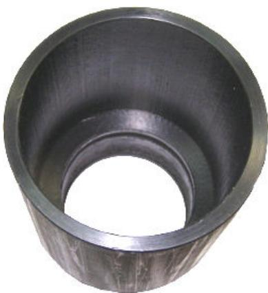
Figure A.8 - Calibration cell for calibration and adjustment of submersible sensors
