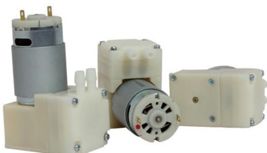
Figure A.11 - Compressor for cleaning submersible sensors (12 VDC, 0.6 A, pressure up to 1.5 bar, air flow up to 4 l/min, dimensions 74 × 51 × 32 mm)
