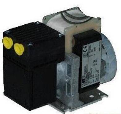
Figure A.10 - Compressor for cleaning submersible sensors (~ 220 VAC, 60 W, pressure up to 2.4 bar, air flow up to 6 l/min, dimensions 103 × 93 × 64 mm)
